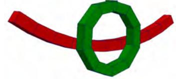
Figure 2: green: without shear locking, red: with shear locking
